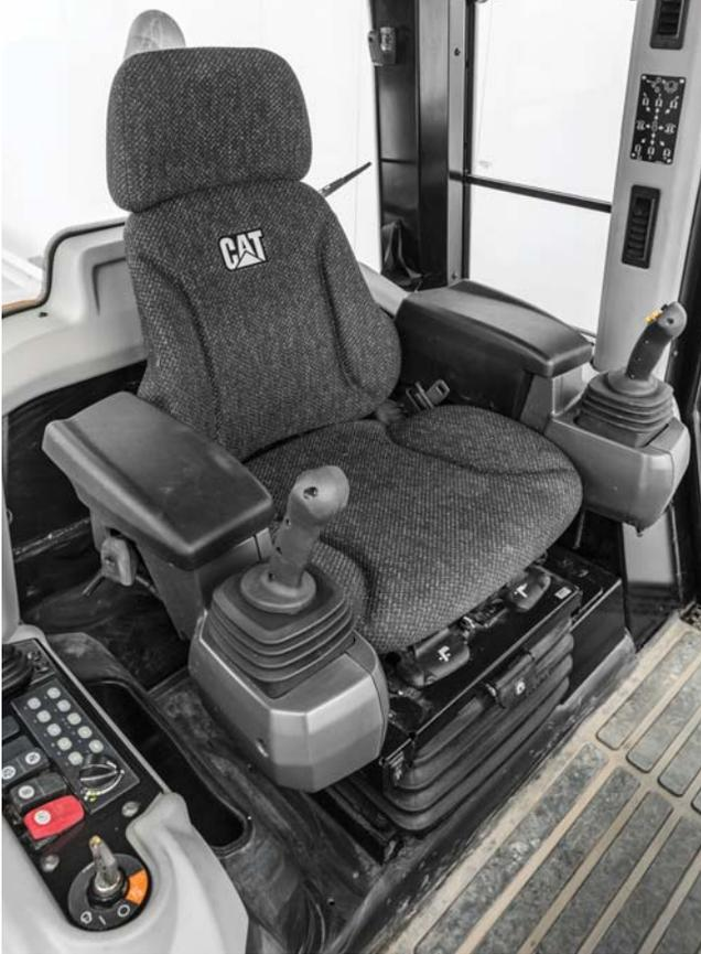
Updated cab gives operators added comforts like adjustable armrests and controls, improved air conditioning system and a heated/ventilated seat option. The Liquid Crystal Display (LCD) operator interface makes it simple to customize machine performance features and to view machine operating and service information.
